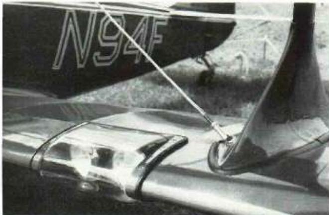
The landing and taxi lights are enclosed in a blown protective lens. Rubber booting surrounds this as well as the interplane strut cuffs. Note the way in which the flying wire clevis goes into the cuff.
