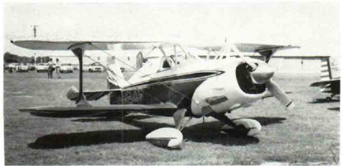
A first impression is that the "Mirage II" has a radial engine because of the large cowl and frontal opening.
